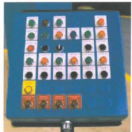
Trim Press Operator Interface
