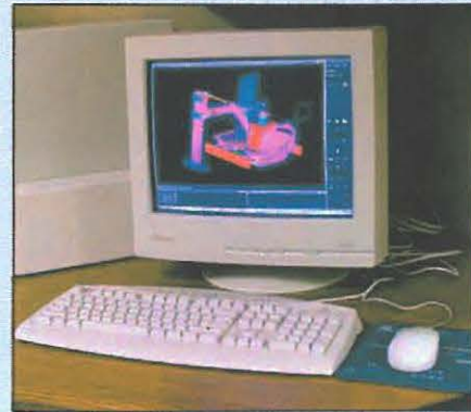
SDRC Ideas 3-D solid modeling program is used to design the sprayer.
